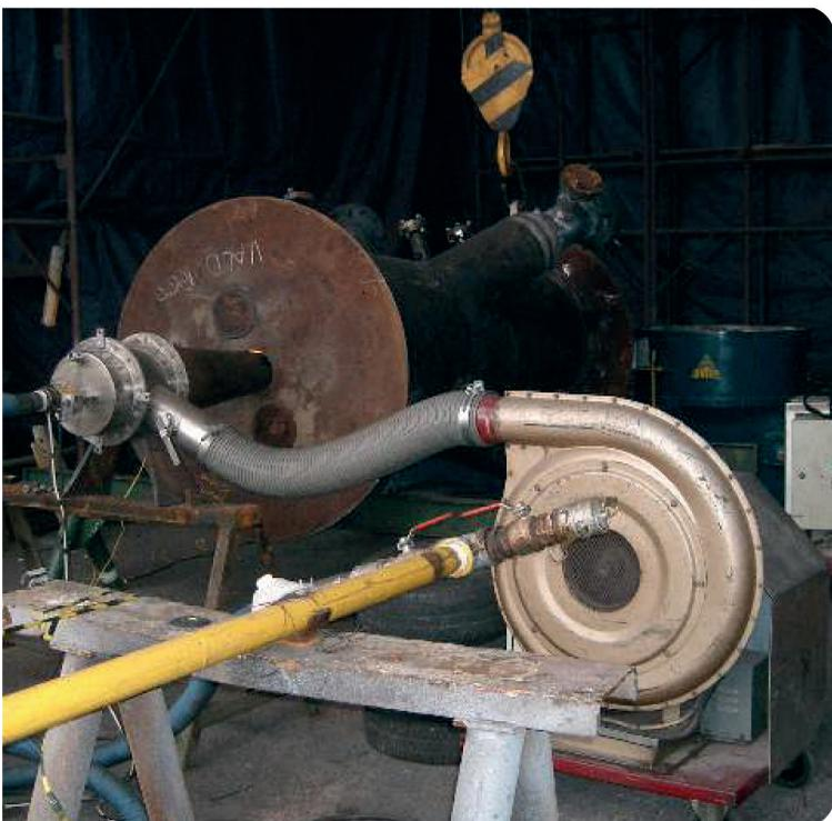
Tecnotrat has portable equipment consisting of high-speed gas burners with convective heating method, it can work with natural gas and LPG.
