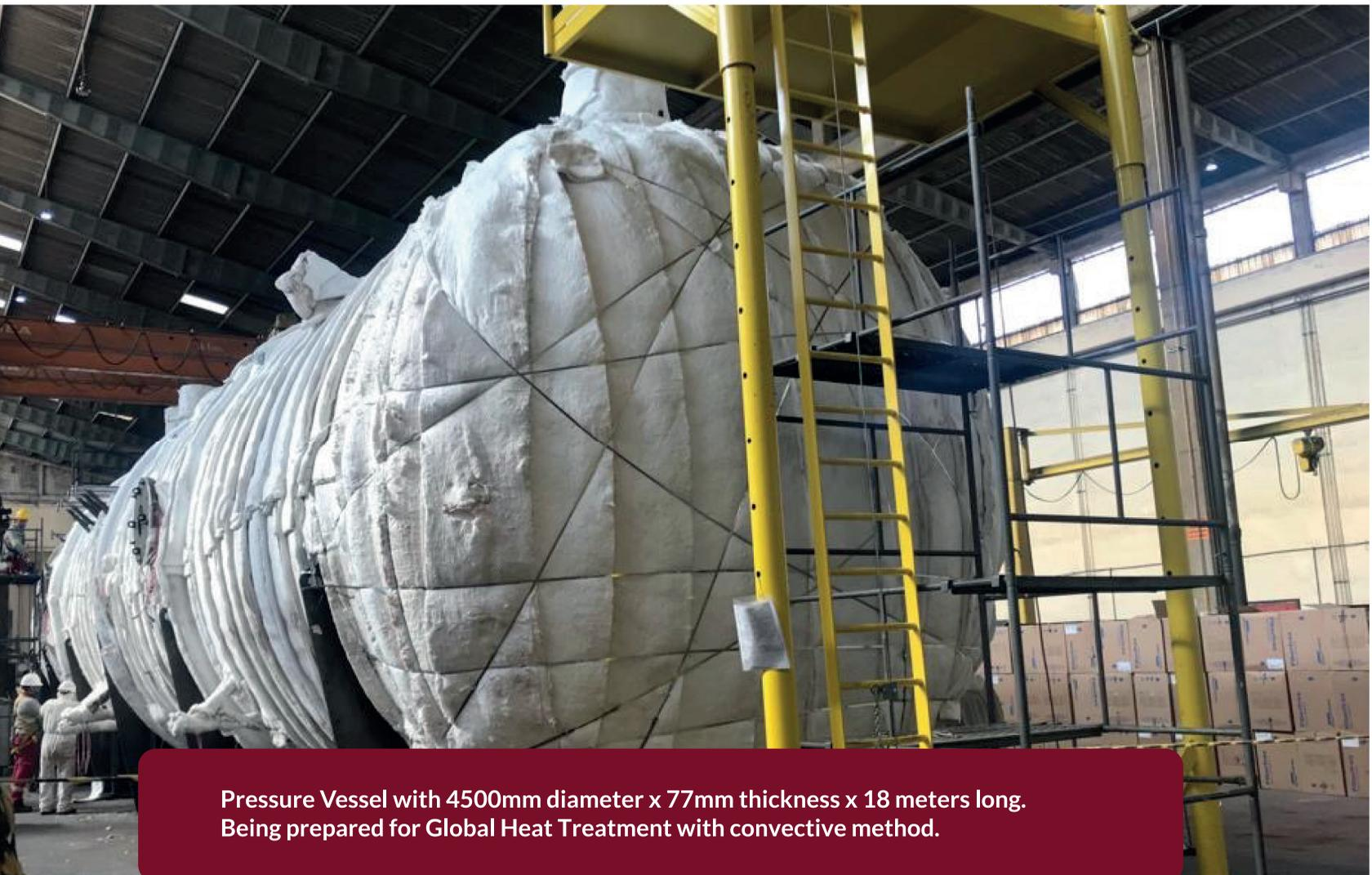
**Pressure Vessel with 4500mm diameter x 77mm thickness x 18 meters long.
